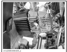
UNSCREW SPARK PLUG ONE TURN 1. Spark plug
